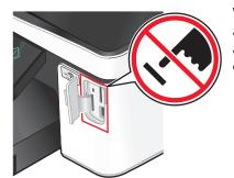
**Warning—Potential Damage:** Do not touch any cables, any network adapter, any connector, the memory device, or the printer in the areas shown while actively printing, reading, or writing from the memory card. A loss of data can occur.
