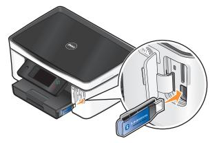
Bluetooth Dongle Connected appears on the display.
