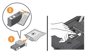
**Note:** Install the new ink cartridges immediately after removing the protective cap to avoid exposing the ink to air.
