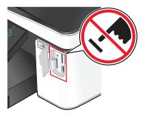
**Warning**—**Potential Damage:** Do not touch any cables, any network adapter, any connector, the USB Bluetooth adapter, or the printer in the areas shown while actively printing, reading, or writing from a Bluetooth-enabled device. A loss of data can occur.
